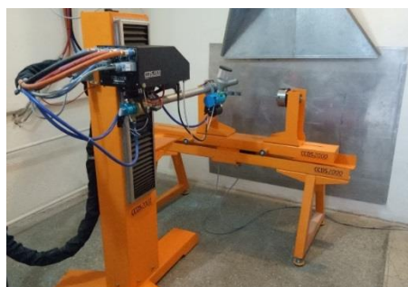
Figure 1. Diagram of the detonation spraying unit "CCDS-2000"
