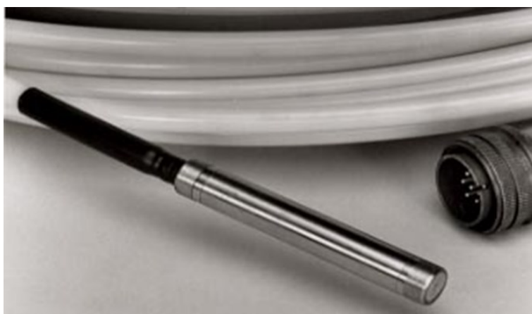
Figure 2. Internal MFL probe for finfan tube inspection
