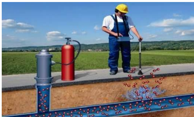
Figure 4. Water leak detection device using indicator gas
