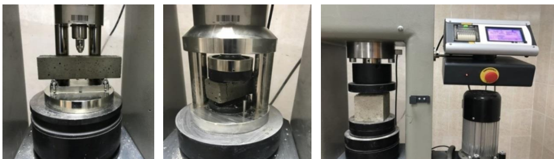
Figure 1. Bending and compressive strength tests
