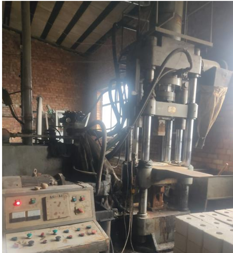
Figure 1. Press for making salt briquettes-licks
