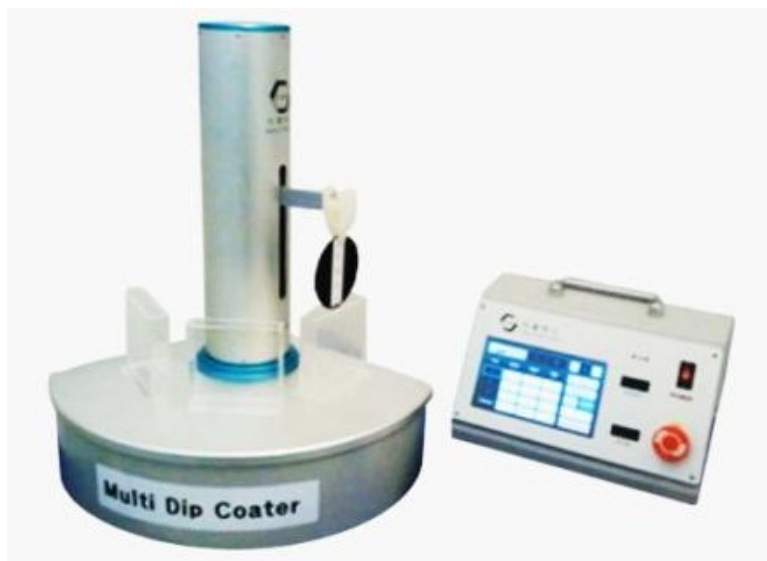
Figure 5. Photographic image of the installation for carrying out dip-coating synthesis
