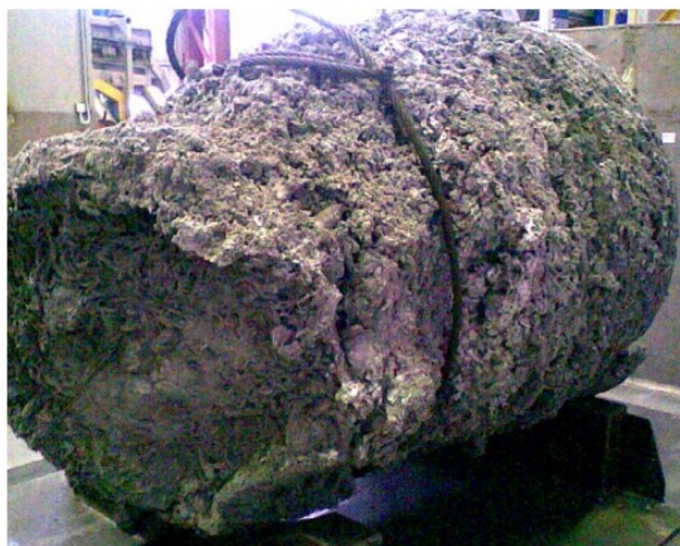
Figure 7. Sponge titanium block weighing 7 tons produced by UKTMC JSC
