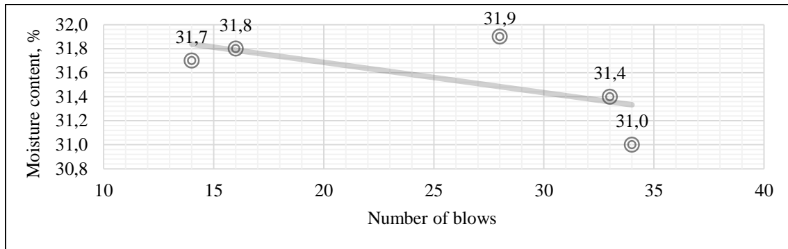
Figure 1. Liquid limit diagram of the soil 1
