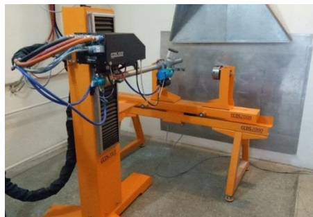
Figure 1. Diagram of the detonation spraying unit "CCDS-2000"
