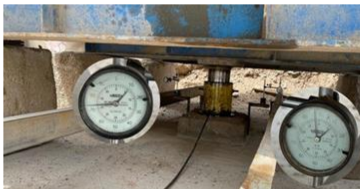
Figure 4. Dial gauges' readings during 150 Tons load test
