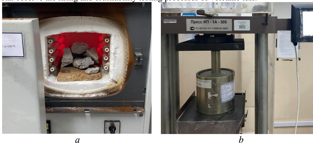
Figure 1. a) firing of volcanic tuff in a muffle furnace; b) crush testing of volcanic tuff on a hydraulic press
