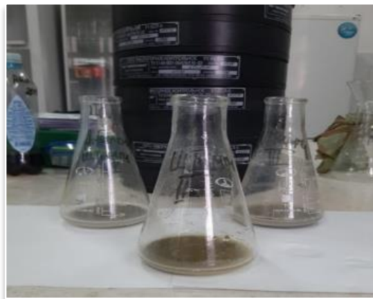
Figure 3. Adsorption of A. Ferrooxidans cells on the surface of ore minerals by static adsorption
