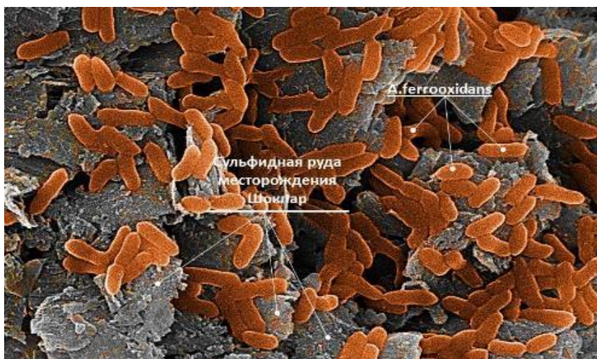
Figure 5. Adsorption of A. ferrooxidans bacteria cells on the surface of ore particles of the Shokpar deposit
