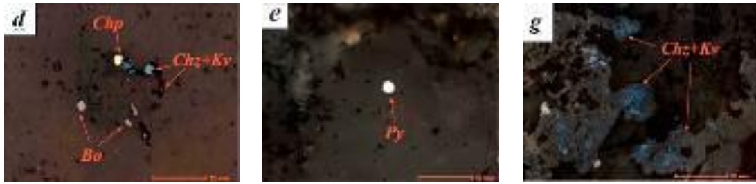
Figure 4. Polished section: a-g – amygdules composed of grains of chalcocite and covellite; d-e – single grains of chalcopyrite, pyrite and bornite
