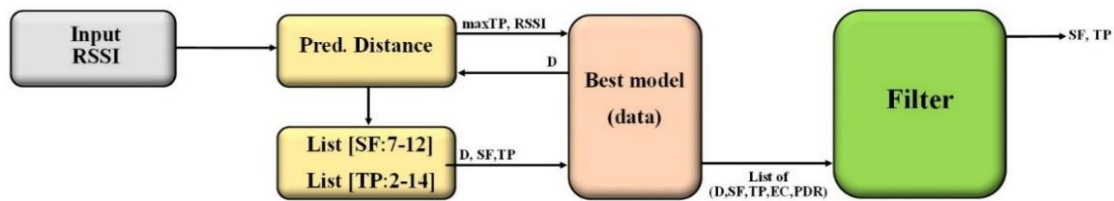
Figure 4. Algorithm for optimizing SF and TP parameters
