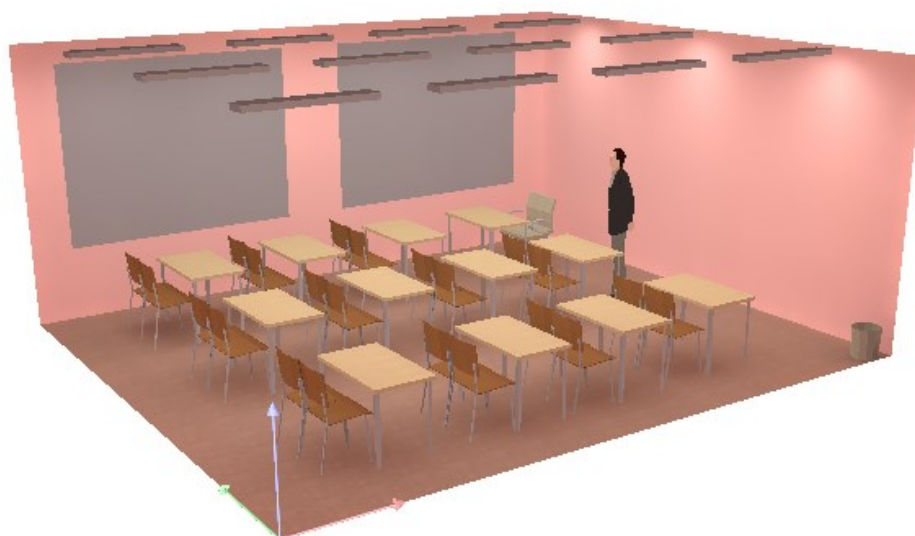
Figure 2. Model of LED lighting of the classroom using LEDEL L-school 32 luminaires
