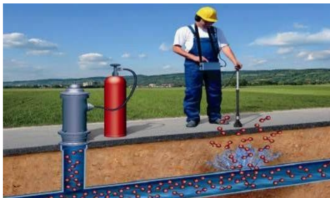
Figure 4. Water leak detection device using indicator gas
