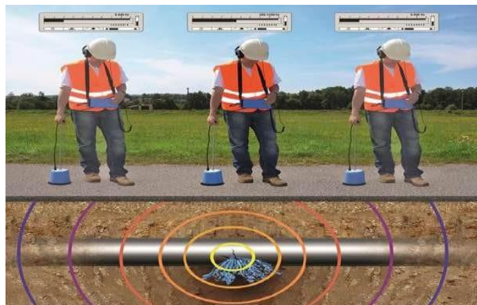
Figure 1. Method of acoustic leak detection in water pipes
