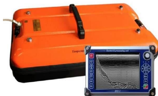
Figure 3. Portable GPR for water leak detection
