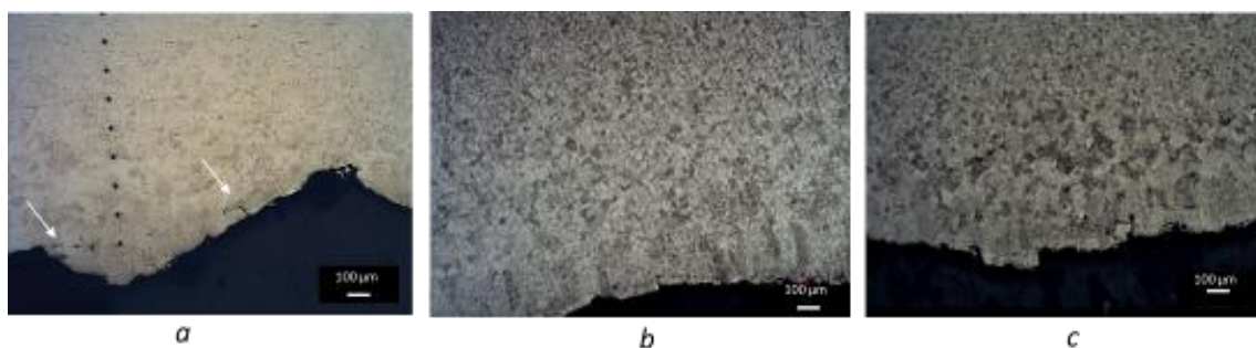
Figure 2. Hardened 65G steel layer by electrofriction treatment at speeds: 0.83 rpm (a), 1.33 rpm (b), 2 rpm (c)
