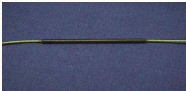
Figure 6. FBG temperature sensor [10]
