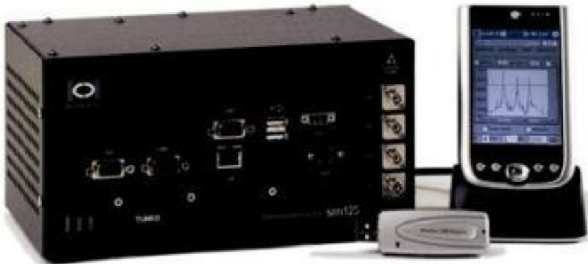
Figure 1. View of SM125 optic sensor interrogator's front [5]
