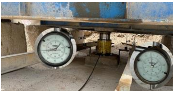
Figure 4. Dial gauges' readings during 150 Tons load test
