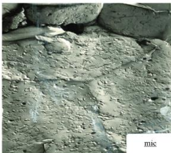
Figure 10. Fractogram of a fracture of a sample of hot-pressed beryllium PTB-56 with inclusions of beryllium oxide
