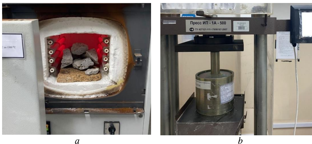
Figure 1. a) firing of volcanic tuff in a muffle furnace; b) crush testing of volcanic tuff on a hydraulic press
