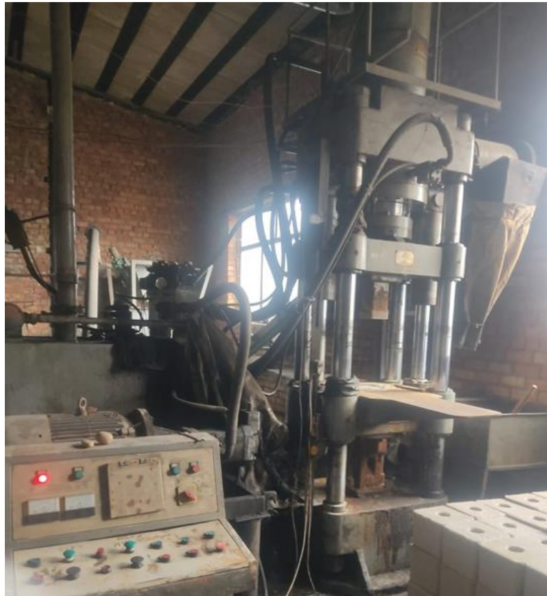
Figure 1. Press for making salt briquettes-licks
