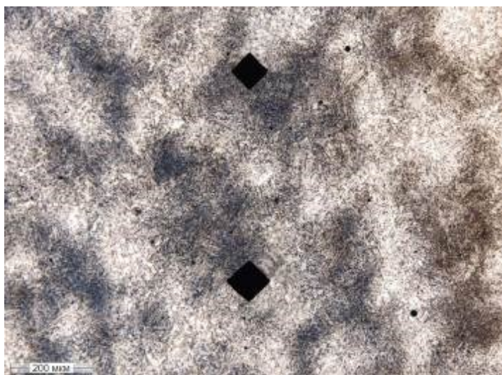
Figure 8. Microstructure of the 42XMFA steel sample surface after EPT
