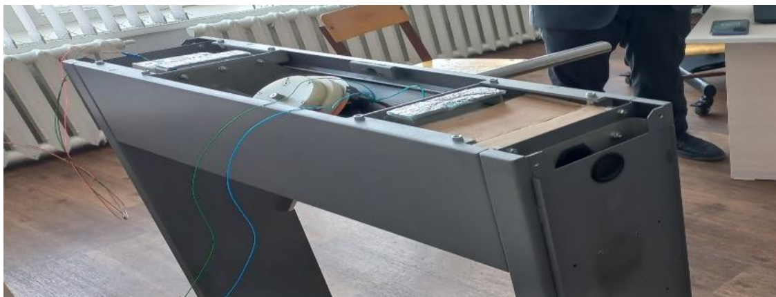
Figure 1. Turnstile, automatic rotation of the blocking slats is carried out due to the built-in electric drive
